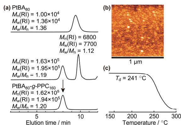
Figure 1. (a) GPC traces of PtBA<sub>80</sub> (top), product after CO<sub>2</sub>-PO copolymerization (middle), and PtBA<sub>80</sub>-*g*-PPC<sub>160</sub> (bottom). (b) AFM image and (c) TGA curve of PtBA<sub>80</sub>-*g*-PPC<sub>160</sub>.
