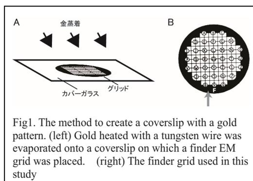
Fig1. The method to create a coverslip with a gold pattern. (left) Gold heated with a tungsten wire was evaporated onto a coverslip on which a finder EM grid was placed. (right) The finder grid used in this study
